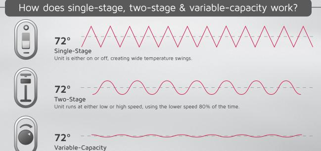
Unit runs at low most of the time, using only the amount of energy necessary to meet comfort need.
